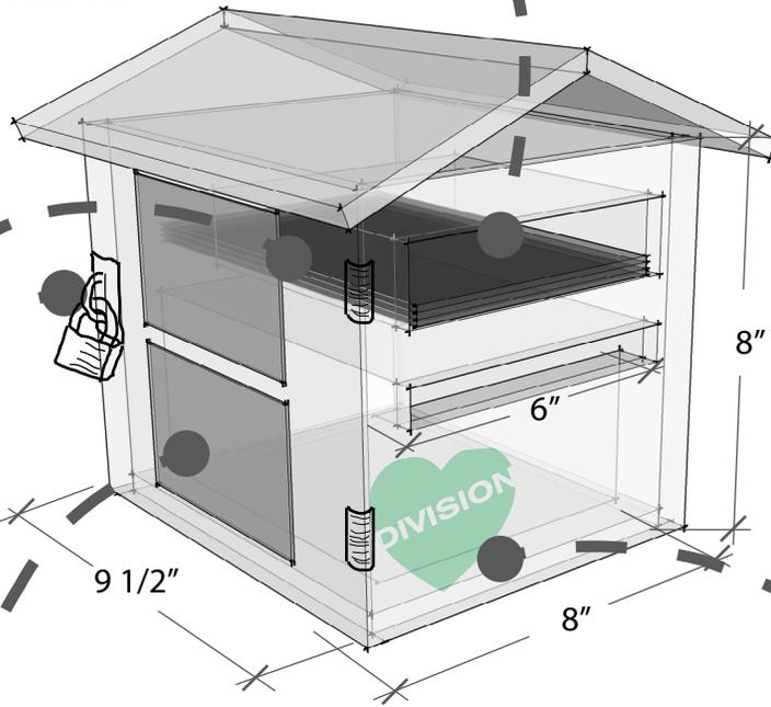
One side of box should have a hinged panel with option to lock to keep submissions secure until collected.
