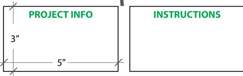
Project Info and Instruction cards need to be visible on sides (or front) of box. They are separated into two panels for flexibility on installation location. They could be attached next to each other as shown or one on each side.
